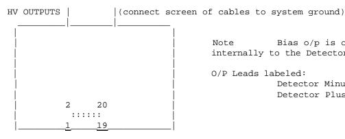
Note Bias o/p is connected internally to the Detector Negative.
